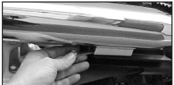
Figure 5. Installing the nut plate on the muffler body.
